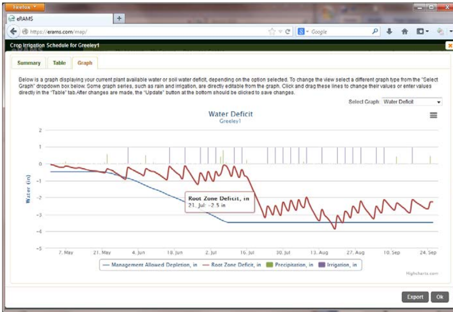
Figure 5. Example graph showing daily water deficits in the root zone (red line; inches of water) in relation to management allowed depletion (MAD, blue line). Irrigation is recommended when the red line approaches or falls below the MAD. Daily precipitation and irrigation are also shown as vertical bars in the graph.
